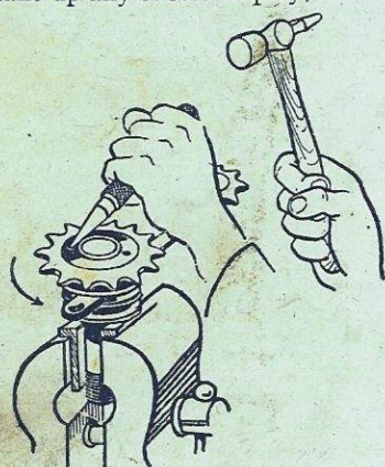
Removing the end plate from the operating cog to take up end play by shim removal
