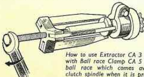
The Extractor for the ball race on the valve side of the crankshaft (Service Tool CA 4) shown in use with the Ball race Clamp (Service Tool CA 5). See page 22, para. 26.
