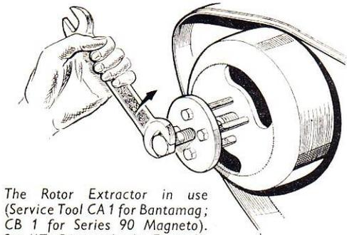
The Rotor Extractor in use (Service Tool CA 1 for Bantamag; CB 1 for Series 90 Magneto). See "To Dismantle the Engine", page 22, para. 8.
