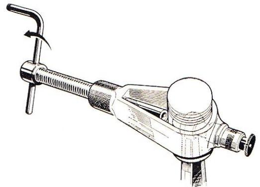
The locating fitment shown is supplied with the Piston and Gudgeon Pin Tool (CA 10 is illustrated) for use when refitting piston to con-rod. The pin of the fitment serves as a mandrel to locate the little end in position, and its length is such that it serves as a stop to prevent further movement when the gudgeon pin is properly home. CB 10 is an alternative tool which fits both pistons. See "Before Re-building the Engine," page 23.
