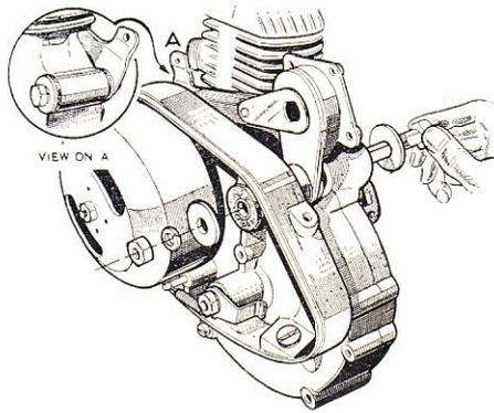
Removing the engine suspension bolts. See page 6.
