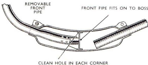
1. Remove complete exhaust system and clamping screw where exhaust pipe enters silencer (in a few cases there is no screw—it is a push fit).
