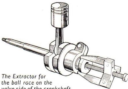
The Extractor for the ball race on the valve side of the crankshaft (Service Tool CA 4) shown in use with the Ball race Clamp (Service Tool CA 5). See page 22, para. 26.
