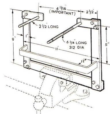
The straightforward framework shown in this illustration is indispensable for dismantling and reassembling the engine.
