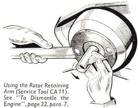
Using the Rotor Retaining Arm (Service Tool CA 11). See "To Dismantle the Engine", page 22, para. 7.
