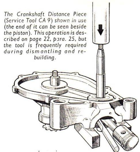
The Crankshaft Distance Piece (Service Tool CA 9) shown in use (the end of it can be seen beside the piston). This operation is described on page 22, para. 25, but the tool is frequently required during dismantling and re-building.
