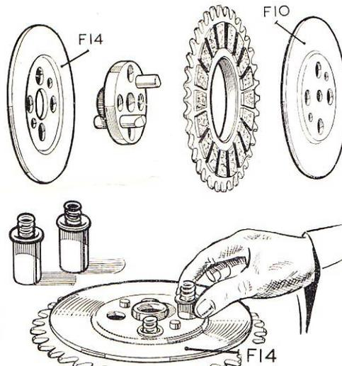
The correct way to assemble the clutch. See page 26, para. 15.
