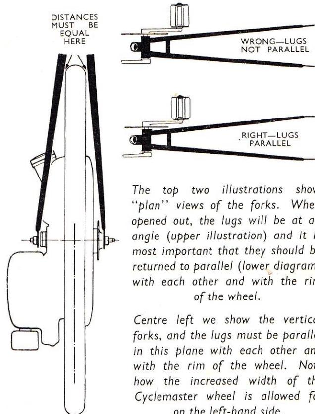
The top two illustrations show "plan" views of the forks. When opened out, the lugs will be at an angle (upper illustration) and it is most important that they should be returned to parallel (lower diagram) with each other and with the rim of the wheel.
