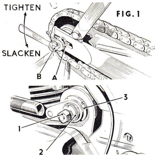
The two illustrations above show the method of adjusting the New Eadie Coaster Hub. Nut 2 is not fitted on some wheels. Nut 3 is used only for adjusting tension of chain from clutch to drum. (See page 5.)
