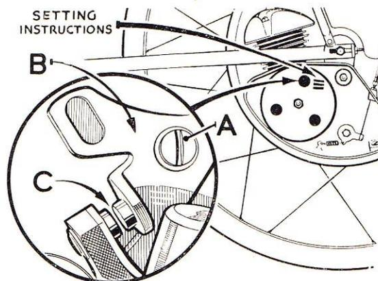
How to inspect and adjust the contact breaker points on Wheels No. 1 to 76750. To adjust the points; slacken screw A and move the plate B as necessary to open or close the points C. When correct tighten A and recheck.
