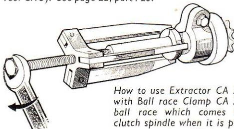
How to use Extractor CA 3 in conjunction with Ball race Clamp CA 5 to remove the ball race which comes away with the clutch spindle when it is pressed out. See page 22, para. 28.
