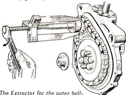
The Extractor for the outer ball race on the driving side of the crankshaft (Service Tool CA 3). See "To Dismantle the Engine", page 22, para. 16.
