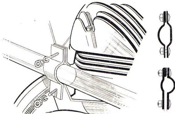
The correct fitting of the engine locating bracket is most important. Brackets for both "D" section and "O" section forks (as illustrated) are available.
