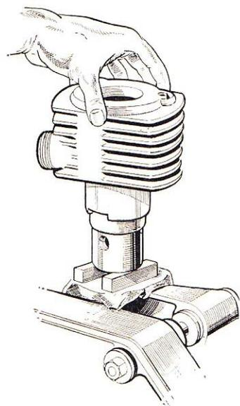
The use of the Piston Ring Sleeve (Service Tool CA 8 for 25.7 c.c. engines, CB 8 for 32 c.c. engines). See page 26, para. 30.
