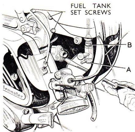
Removing the B.E.C. carburettor from the engine. In this drawing the fuel tap nipple has had to be shown pointing the wrong way.
