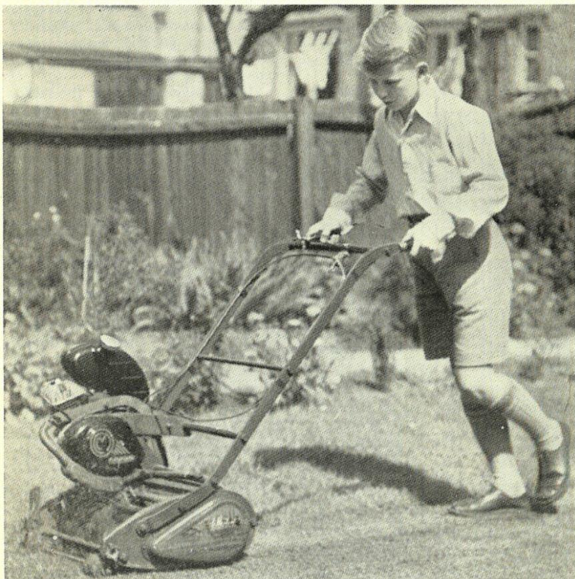
A reader in Harrow sent us this photograph showing his "Cyclemaster" powered lawn mower. He says it has taken the hard work out of mowing and can be used when the ground is too wet to use a hand pushed mower. The mower itself gave several years reliable service before being converted to power drive, but the original bearings of the cutter cylinder do not appear to be heavy enough to satisfactorily take the added strain. Modifications are being made to overcome this difficulty
