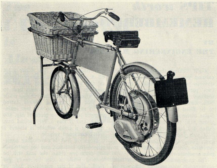
A photograph of the Cyclomaster Roundsman, which carries a payload of 1 cwt. Advertising plate, licence holder, number plates and stand are included in the price. Basket, lamps and wiring are optional extras
