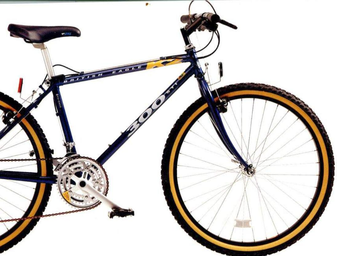
**K 2** Reynolds 501 all terrain tubing. Shimano Exage 21 speed 300 CX, three finger rapid fire gears and short reach Low Profile brakes. Exage Biopace chainset.
