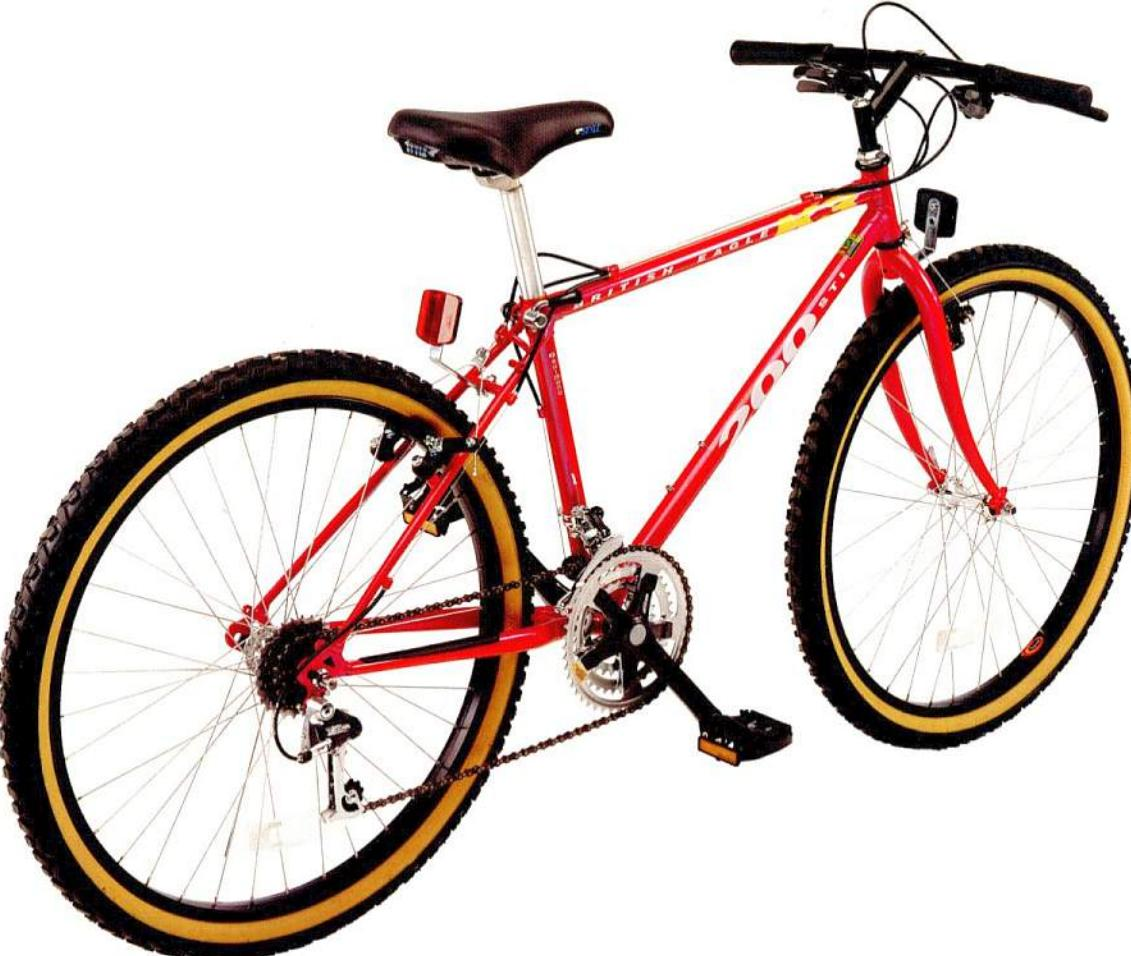
**K 3** Reynolds 500 all terrain tubing, Shimano Exage 200 rapid fire gears and Low Profile three finger brakes.
