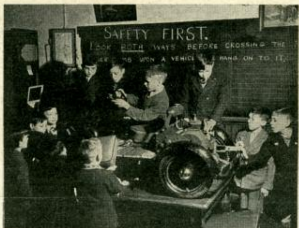
By undoing 12 nuts, the body of the Atco trainer can be removed, leaving the chassis clear for use as a lecturing model in the classroom
