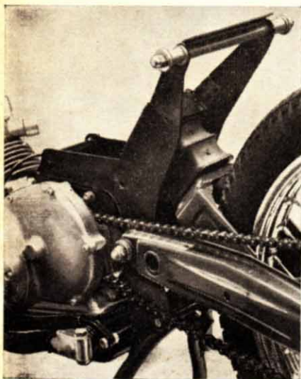
A rubber block takes road shocks at the rear. The fork is pivoted on grease-packed nylon bushes
