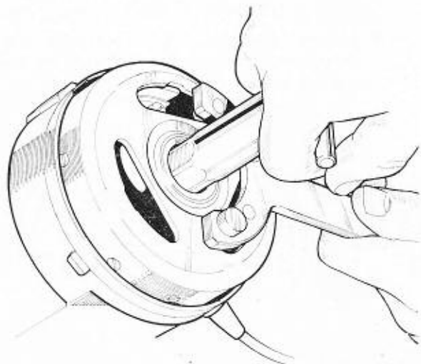
FIG. B11. Releasing flywheel nut.
