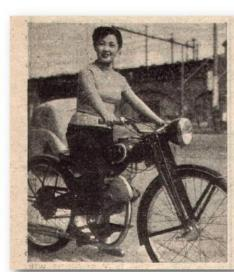
Ultra - lightweight— Nippon-style, This autocycle from Japan, the Arai "Terrie" has an 88 c.c. o.h.v. engine and is made by Arai Auto Co. Ltd., of Tokyo.
