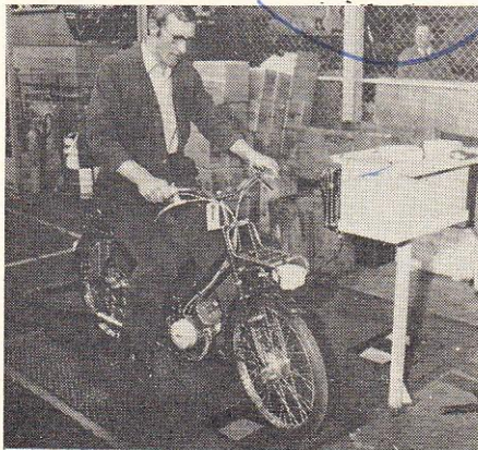
All the machines are roller tested before leaving the factory. Engines are also separately tested following assembly.
