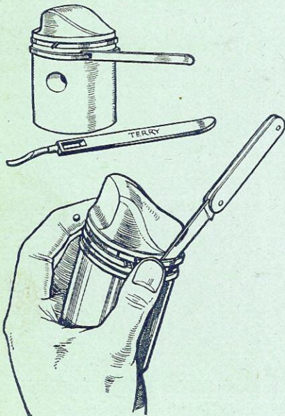
Alternative method of piston ring removal.
