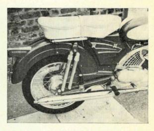
Rear suspension units can be used together or separate. The pump under the saddle is standard
