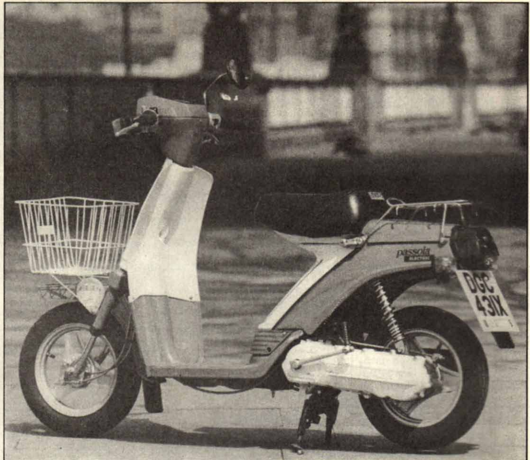
Pretty little Passola uses restricted 50cc single-cylinder, two-stroke motor giving only 2.8bhp
