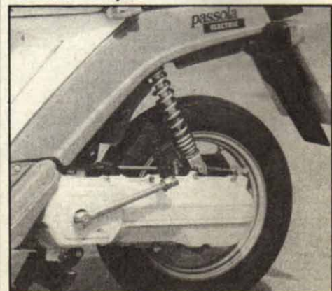
Chain final drive is fully enclosed; single damper at rear
