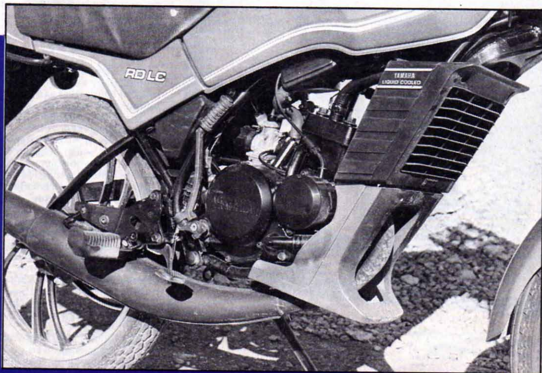
Liquid cooling allows the single cylinder two-stroke engine to develop almost 9bhp with a 10,000rpm redline.
