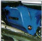
Yamaha's world-famous Autolube injection precisely controls the supply of oil to the engine ending messy has and oil mix. Improves engine operation and saves oil and gas. Drastically
