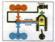
No pre-mixing of oil and gas is necessary. Both the gasoline and the oil are separately sent to the engine, where they are regulated automatically and with extreme accuracy to supply exactly the correct mixture. Features: No gasoline/oil mixing \*Engine oil stays clean \*No engine overheating.... engine stays clean \*No smoke and no carbon \*Less engine trouble and longer service \*No troublesome engine adjustment....maintenance costs are lower \*Smooth starts and fast acceleration.
