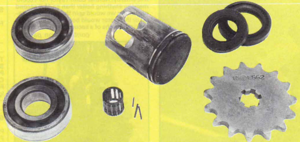
Above: Piston, small end bearing, main bearings and oil seals were reduced to scrap.
