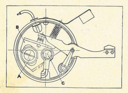
The complete condenser box assembly is interchangeable with the type previously fitted, but when ordering, the number of the engine for which it is required should be stated.
