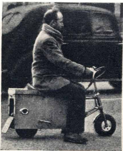
The small wheels and compact dimensions of the Bouffort scooter are apparent from this photograph. Note the hinge-down rear number plate
