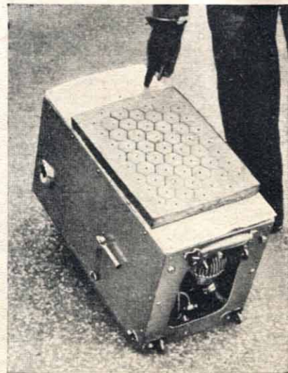
The handlebar and steering assembly can be stowed inside the box which can then be wheeled along by the handle seen in front of the seat cushion
