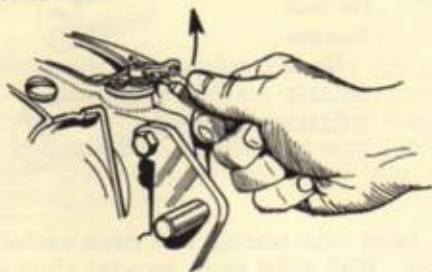
Replacing spring on Gear Change Lever
