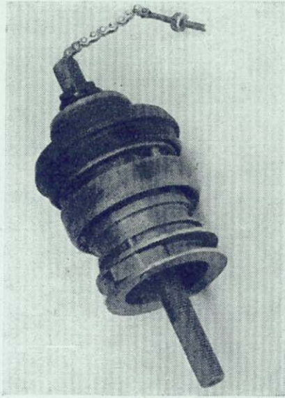
The hub assembly as it appears immediately after removal from the shell
