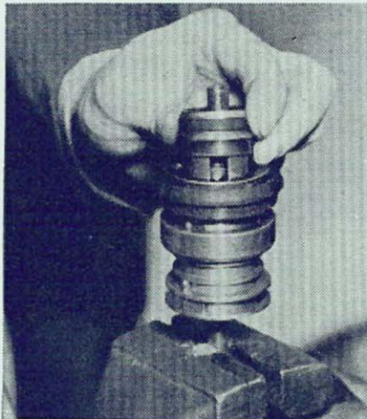
BUILDING UP —The drive dog is being placed in position
