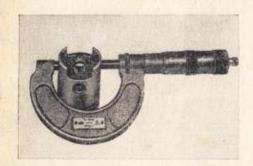
The measurement of the effective diameter is taken at a distance of 10 mm from the lower edge of the piston skirt. When the actual dimension falls 0.1 mm below the nominal diameter, then the piston must be replaced by a new one.
