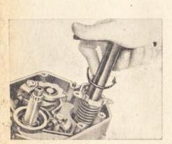
Fit the tensioning plate in such a way that the small pair of the offset lugs points downward and centres the kick-starter spring; the wide one of the three lugs pointing upwards must point to the rear when the kick-starter spring is not tensioned.
