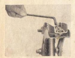
Remove the M8 nut (together with spring ring B8 and lower pressure member) of the carriage bolt M 8 X 43 and draw out the carriage bolt.
