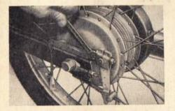
The stop light is adjusted with the help of an open-ended spanner without loosening the check nut. The shaft is turned by means of an open-ended spaner, width over flats 8, until the stop light flashes up. If necessary, the contact must be readjusted in the interior. Checking is effected by actuating the pedal brake while the engine is running.
