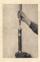
Remove the dust wiper from the slide tube, clamp the foot of the bar carefully and-vertically in a vice. Pull the carrying tube upwards to its final position and remove the snap ring 25 from the lower end of the carrying tube. Pull off the carrying tube upwards.
