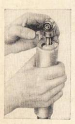
Press down the upper protective sleeve for some distance and remove the semicups.
