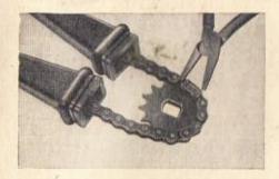
Insert the chain connector opposite to the chain sense of rotation into the grooves of the locking pins.
