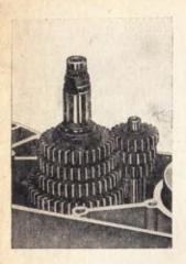
In a 4-speed gearbox, place the thrust washer Ø 10.5/18 mm (1 mm thick) on the gear for the 4th speed.
