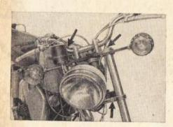
Remove the fastening screws M  $8 \times 30$  from the top fork guide and loosen the clamping screws M  $8 \times 25$  from the lower fork guide.
