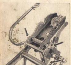
Unhook the brake linkage and the return spring.
