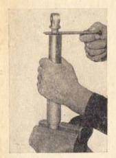
Clamp the suspension unit in a vice. Compress the supporting spring with the lower protective sleeve and insert the retaining fork EV 8 into the respective recess.
