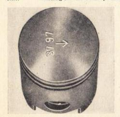
The number stamped in is the piston diameter. The arrow-head indicates the mounting direction of the piston, that is to say, when mounting the piston, the arrow points in the direction of the exhaust port.
