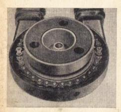
Draw the driving chain into the chain protection hoses and insert the two chain ends into the connecting socket of the chain protection.
