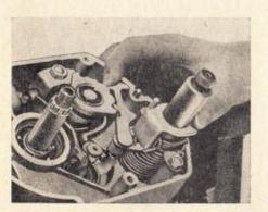
Mount the pre-assembled gearshift lever (consisting of hollow shaft, pawl and torsion spring) in such a way that the gearshift pawl moves past the first and second lock notch of the cam disk on the gearshift cylinder.
