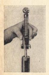
Check the shock-absorber for tightness and signs of wear.
