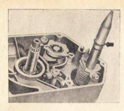
Mount the annular ring  $12 \times 2$  by means of the fitting sleeve "V 014".
