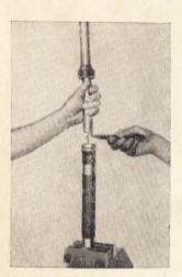
Fit the annular ring and insert it together with the spring holder into the carefully cleaned slide tube which, prior to this, has been provided with the sealing ring D 30  $\times$  40  $\times$  7 (TGL 16454 special design of the internal diameter).
