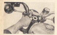
Remove the cable control bushing from the slotted nut at the guide tube and loosen the slotted nut.
