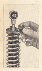
Clamp the suspension unit in a vice. Set the adjusting sleeve to solo operation.
