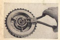
Heat the driver, mount the ball bearing 6203 with an amount of 2 cm<sup>3</sup> of antifriction bearing grease and fit the lock ring, also known as snap ring.
