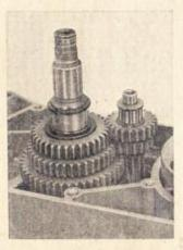
The readily mounted output shaft is now mounted into the left-hand casing half (ball bearing 16004).
