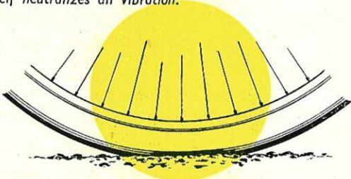
The effect of the Driving Roller is the same as the effect of the road surface.
