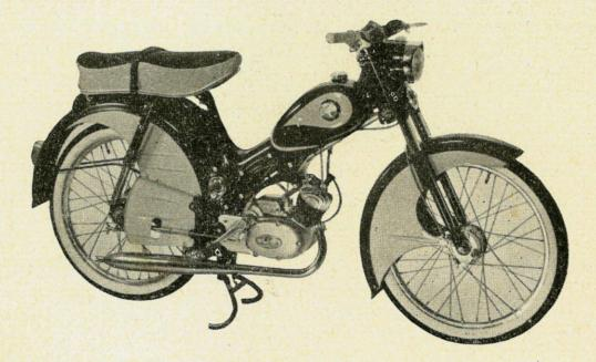
The latest BOBBY 6, 2-seater, re-designed telescopic forks, new shrouded handlebar with built-in lighting and speedo
