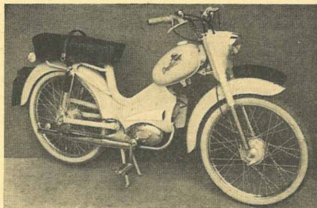
The latest Kerry Capitano de Luxe with three-speed gear box. Robustness, yet simplicity, of frame design is a notable feature
