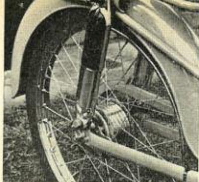
Cam type chain adjusters, full width hub and telescopic spring units can be seen here
