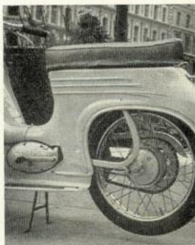
Two coil springs under the saddle control rear forks
