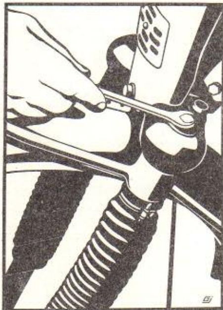
14 - Removal of front telescopic fork
