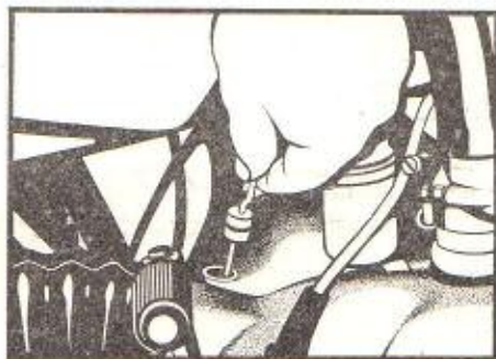
11 – Oil level checking
