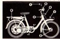
1 Long arm wing mirror, 2 theft-proof steering column lock, 3 spring leading-link front fork, 4 electric horn, 5 speedometer set into headlight, 6 tool kit under the petrol tank, 7 basket mount; you can carry up to 66 lbs between the front and
