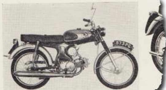
NEW HONDA (above) the 90cc 590 with ohc engine and four-speed gearbox.
