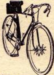
Hercules "Kestrel" OBBU Upright frame, entirely brazed up; Rose pattern forks; Dunlop Sports on 26 in. x 1 1/2 in. Endrieks; adjustable handlebar stem; Hercules front and rear calliper brakes; finished black; usual bright parts Hercules chrome plated. Price £4.18.6 nett cash or on Easy Terms.
