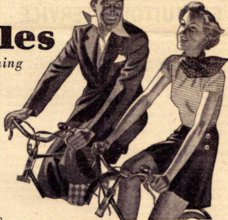
Hercules Safety Model "C" Specially low-built frame, entirely brazed up; short wheel-base; Dunlop Tyres 26 in. x 1 1/2 in.; high raised handlebars; front and rear rim brakes; Hercules spring seat saddle. Price £4.2.6 nett cash or on Easy Terms.
