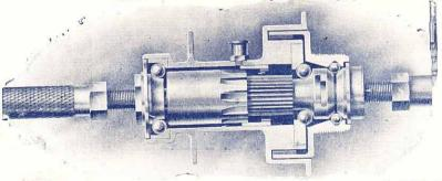
The weight of the rider is not transmitted to the axle through the gearing, there is consequently less friction and an entire absence of those break-downs which occur with other gears.
