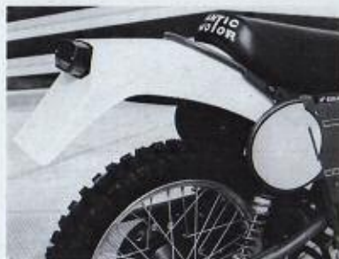
Newly designed mudguard with incorporated tail lamp.
