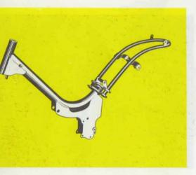
Sturdy monotube framework ensures rigid stability of the whole machine. Plenty of leg-space is allowed by the angle depth in frame and by eliminating a forward placed petrol tank.
