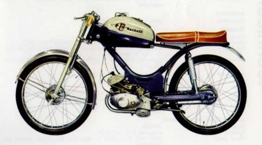
« COMPETITION » engine — 3-speed — special cylinderhead — dell'Orto carburettor dia. 16 mm. — light frame — short handlebar — long saddle — supplied without lighting nor kilometre recorder tyres  $23 \times 2.00$ . accessories: brake pedal and connecting rod for rear brake, cross-
