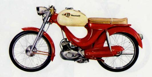
engine: 3 HP. « SPORT » 3-speed. coloured plastic panelling — saddle tank, incorporating tool-box — «Competition» type cap on fuel tank for speedy refilling — long saddle — racing handlebar — kilometre or mile recorder embodied in head lamp — electric horn — long exhaust pipe black tyres  $23 \times 2.00$ . COLOURS: Vermilion framework and cream-coloured tank.
