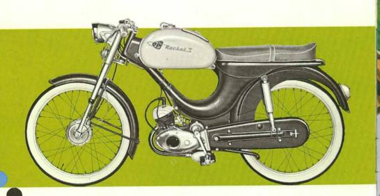
2.2 H.P. «SPORT» engine - front mudguard half-round section - panel type rear mudguard - polyester panelling - saddle tank with incorporated tool-box - «Competition» type cap on fuel tank for speedy refilling - enveloping chainguard - long seat - racing handlebar - kilometre recorder embodied in head lamp - electric horn.
