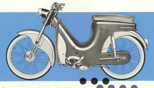
Frame completely enclosed by streamlined panelling in pressed steel plate, 8/10 mm - head lamp embodied in front fork - panelled handlebar with embodied kilometre recorder - opening for inspection of carburettor - panelled mudguards - completely enveloping chainguard with inspection hole - long saddle
