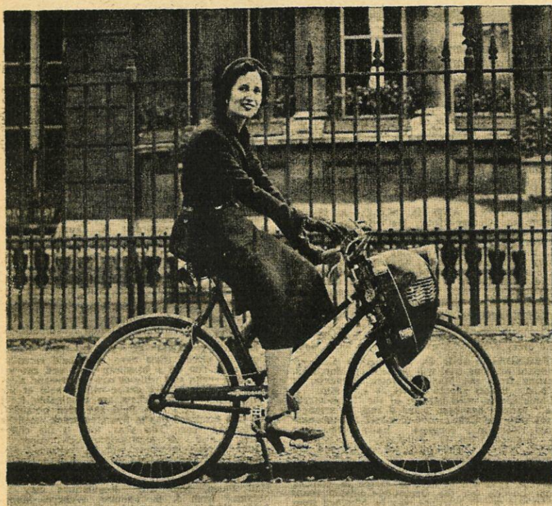
With the power-unit concealed beneath a bonnet, the "Cymota" is an extremely neat attachment which may be fitted to any normal pedal cycle.
