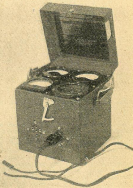
Fig. 5. The completed instrument with test leads, crocodile clips and prods
