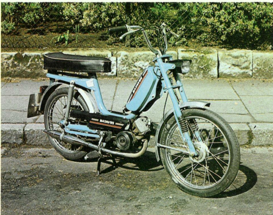
The Batavus Starglo 2 is a single speed automatic pedal assisted moped
