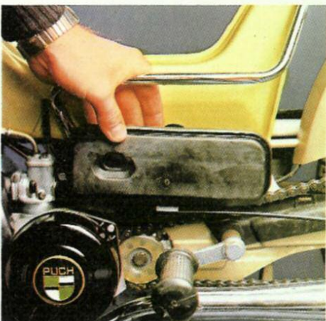
Under the left panel is the air filter which must be cleaned out at intervals of 800 km (500 miles)
