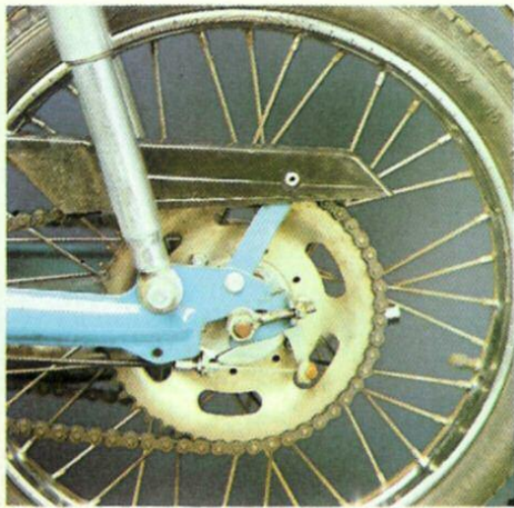
Rear chain adjustment on the Starglo is the same as the Puch. The extra chain has its own tensioner
