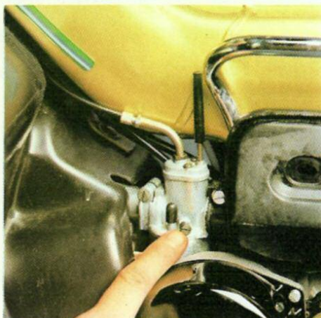
Next to the black tickler button is the throttle stop screw which is turned to adjust the idle speed
