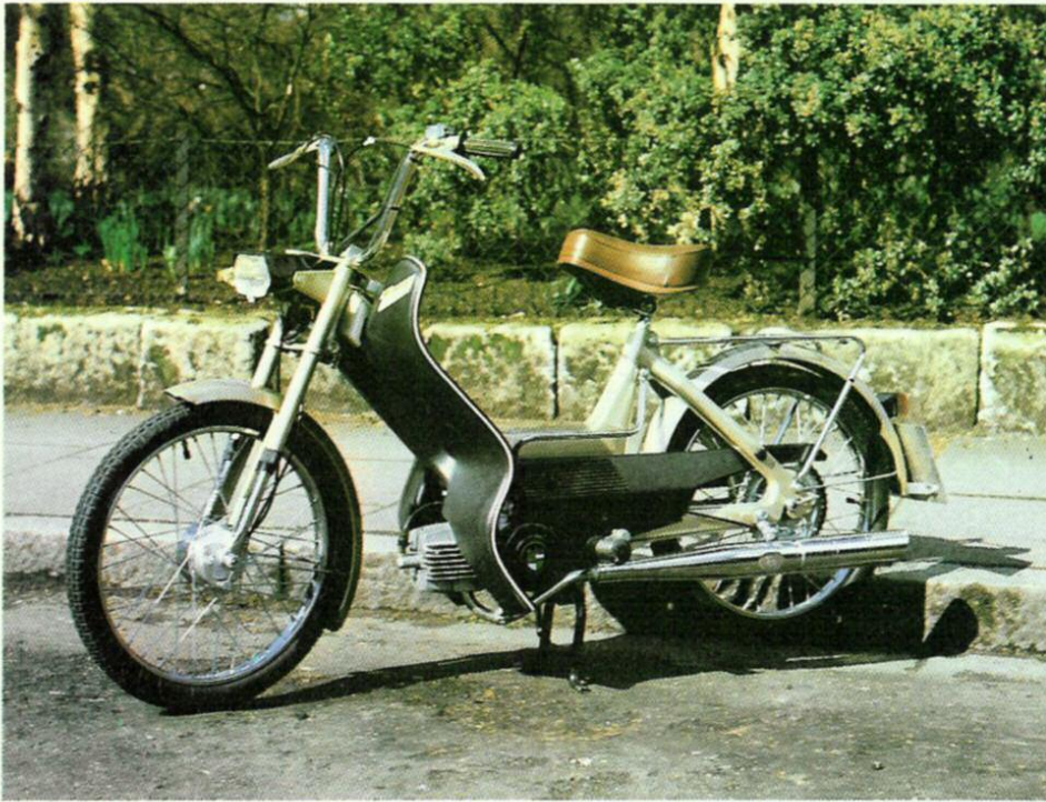
The Puch Maxi Zippy is a single speed automatic, rigid rear end, kick start, pedal-less machine
