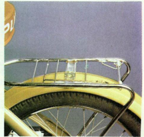
The rear end of the Zippy has a useful chrome plated carrying rack with a spring loaded retaining arm
