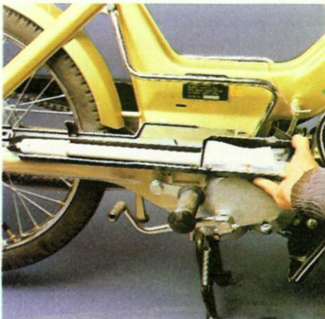
Under the right panel of the Zippy is a very useful tool kit and also a hand pump for the tyres
