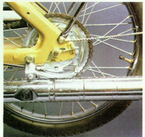
The rear end of the Puch is unsprung. Chain adjustment is made by a simple lock-nutted tensioner
