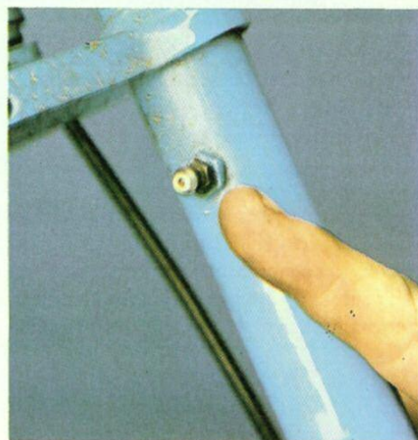
A plus on the Batavus is the front fork greasing point which enables the mechanism to be greased easily
