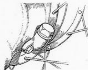
Fig. 4: GEARCASE FILLER PLUG: (rear nearside of unit). Fill with \frac{1}{2} pint (1 \frac{1}{2} filler cap measure) of engine oil (SAE 50).
