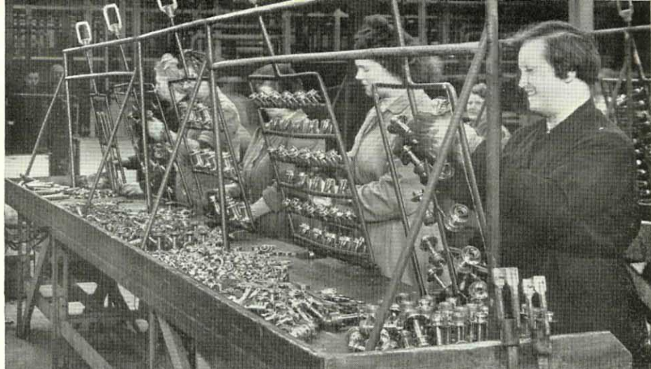
Polished components are loaded on to frame jigs and taken to the plating plant
