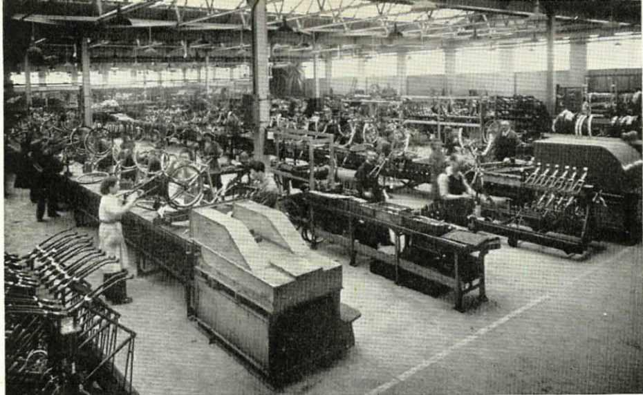
The finished assembly is carried out on the production conveyor lines shown above. Below is the export packing department from where crates of B.S.A. cycles are dispatched to all parts of the world
