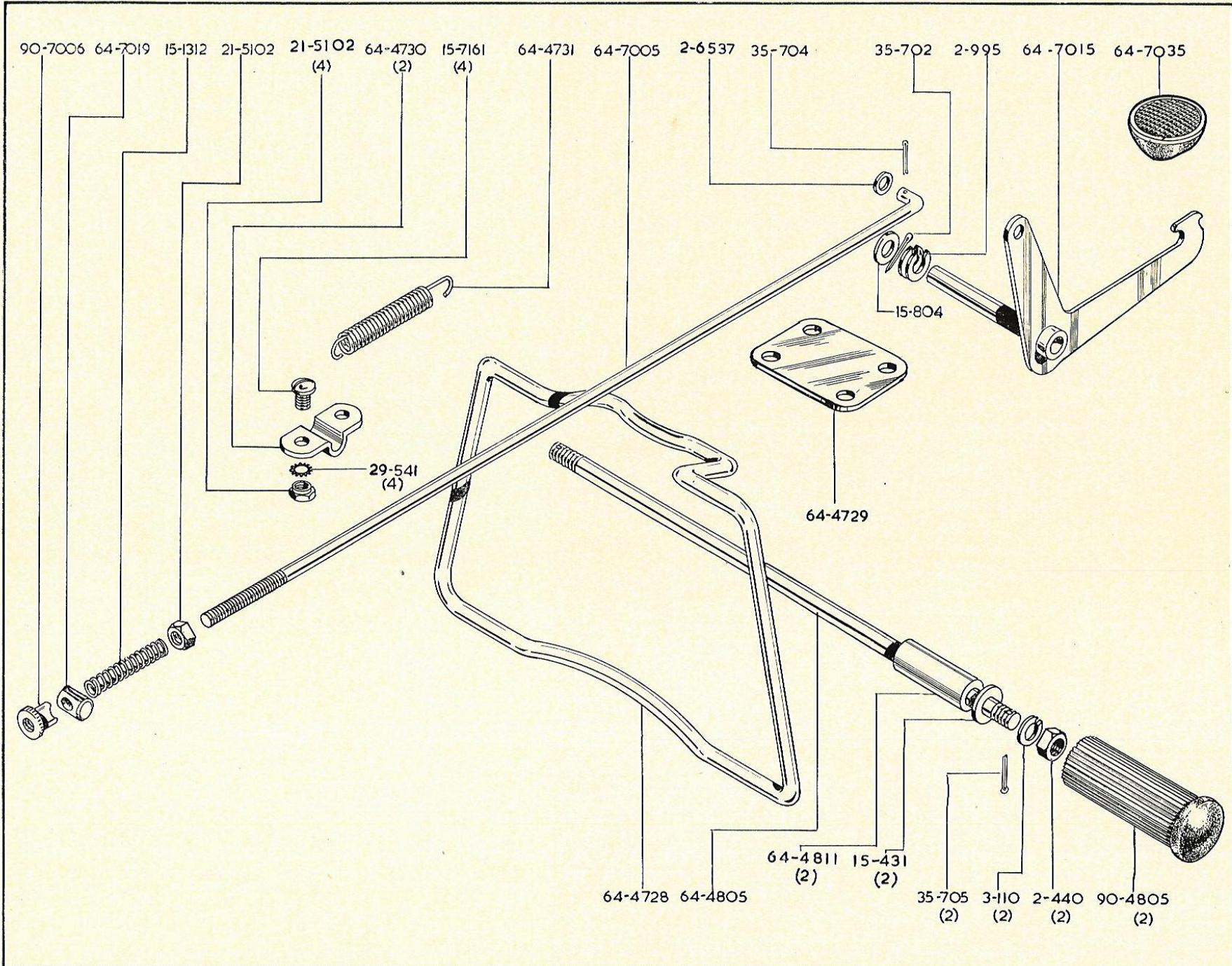
**BRAKE PEDAL, STAND, FOOTRESTS. PEDALES de FREIN, BEGUILLE, REPOSE-PIED
