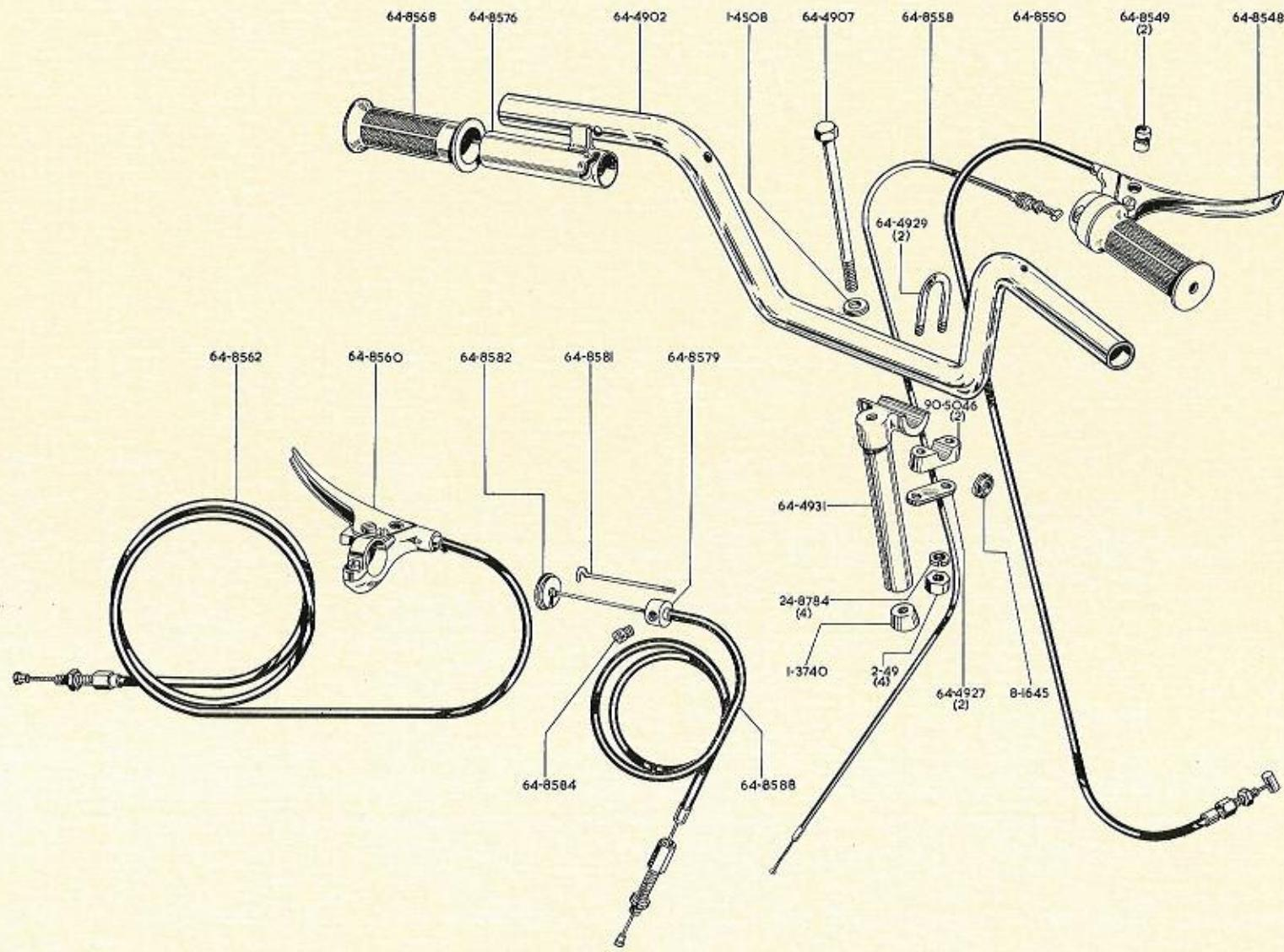
**HANDLEBAR and CONTROLS. GUIDON ET COMMANDES
