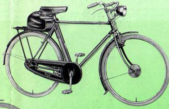
B.S.A. de Luxe Tourist Model 604 ES finished in green with B.S.A. Oilbath, B.S.A. 3-speed Hub with B.S.A. Twist control, roller lever brakes, B.S.A. Hublite, Carrier, Mud-flap and Prop-Stand.
