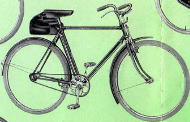
B.S.A. Sports Roadster Model 604 A with roller lever brakes. B.S.A. Sports Roadster Model 604 D with B.S.A. 3-speed Hub.
