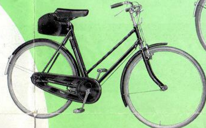
B.S.A. Sports Tourist Model 622 E with B.S.A. Oilbath, B.S.A. 3-speed Hub and roller lever brakes.
