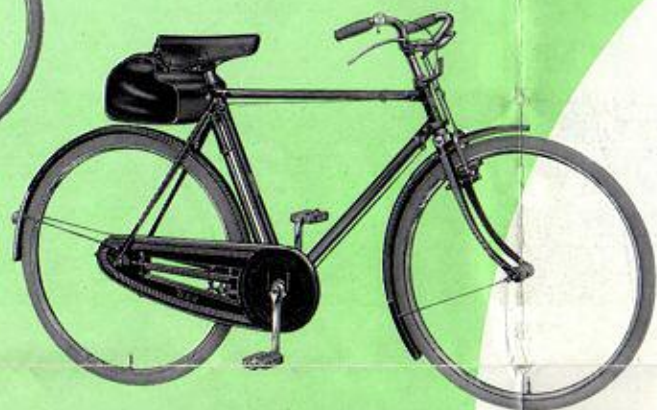
B.S.A. Sports Tourist Model 604 E with B.S.A. Oilbath, B.S.A. 3-speed Hub and roller lever brakes.
