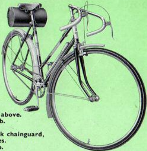
The New B.S.A. Gold Vase 21 1/2 in. and 22 1/2 in. frame of Reynolds 531 tubing; 72° head, 70° seat; patterned lugs, filed; taper seat stays; brazed-on mudguard and pump fittings. D to round fork with solid ends, central in blades, and patterned crown; brazed-on lamp bracket boss. Steering head with inserted race seatings. 26 in. x 1 1/4 in. Endrick rims. Fixed cog and free wheel rear hub. Dunlop Silver Sprite tyres. B.S.A. 5-pin flanged chainwheel, with 6 1/2 in. forged fluted cranks. B.S.A. steel quill pedals. Maes alloy bar on 3 in. steel extension. New B.S.A. side-pull caliper brakes with new B.S.A. levers; silvered cables and plated clips. Ivorette mudguards, spearpoint front. Leather racing saddle. Finish, Flamboyant red with Gold Vase transfers. Metal head badge.
