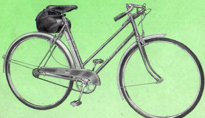
B.S.A. Sports 21 in. and 23 in. frame with taper seat and chain stays brazed-up; forward drop-out rear-ends; brazed on pump pegs. 26 in. x 1 1/4 in. Endrick rims; Dunlop Sports tyres. B.S.A. Maes handlebar, chromium-plated, on adjustable stem; Ladies' model shallow drop. Caliper brakes. Ladies', with reverse action on rear. White steel mudguards, narrow section, front spearpoint with chrome tip. Finish, blue, white lining. Alternative finish Windsor red. Metal head badge.
