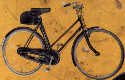
Model 622E with roller lever brakes.
