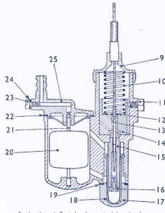
Section through float chamber and mixing chamber.
